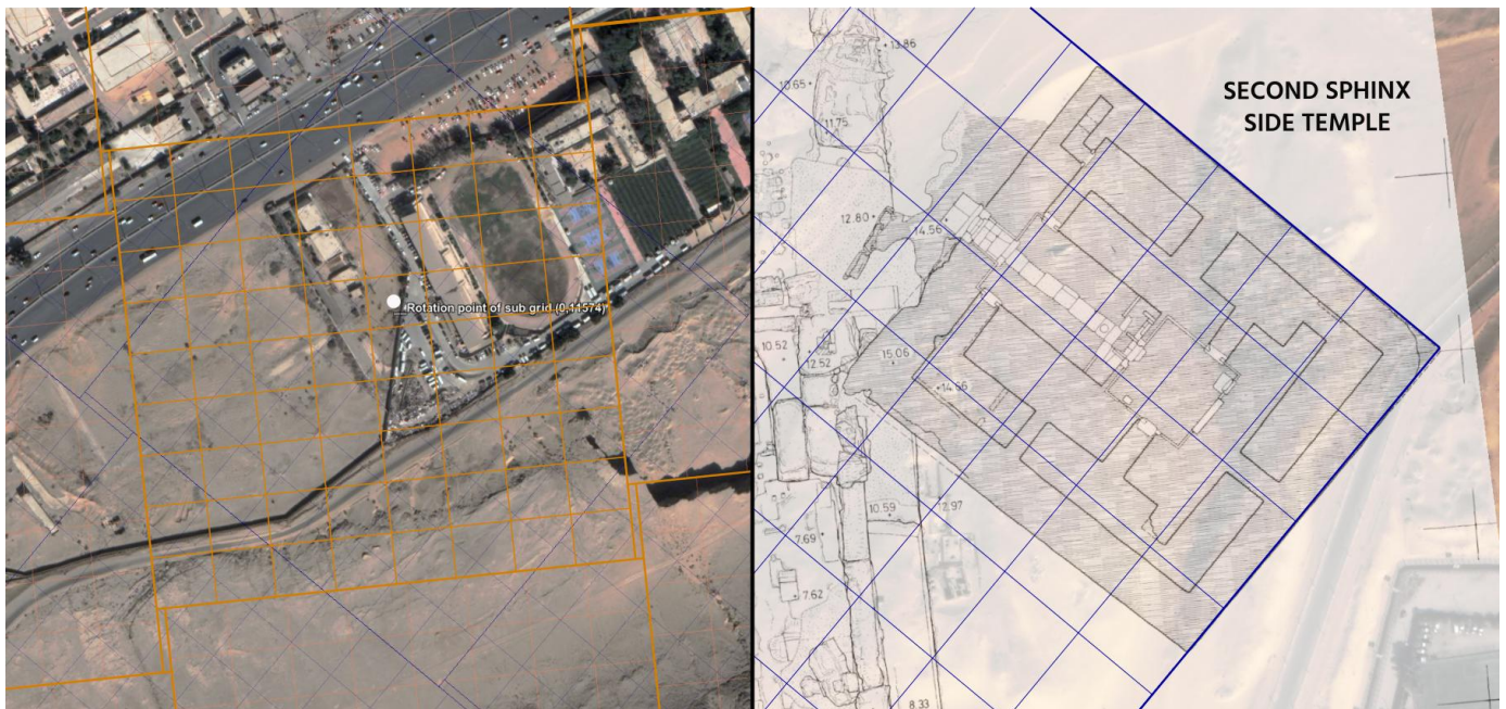
Diagram L60 - The details of the rotation point and the secondary grid alignment of the second Sphinx side temple.
