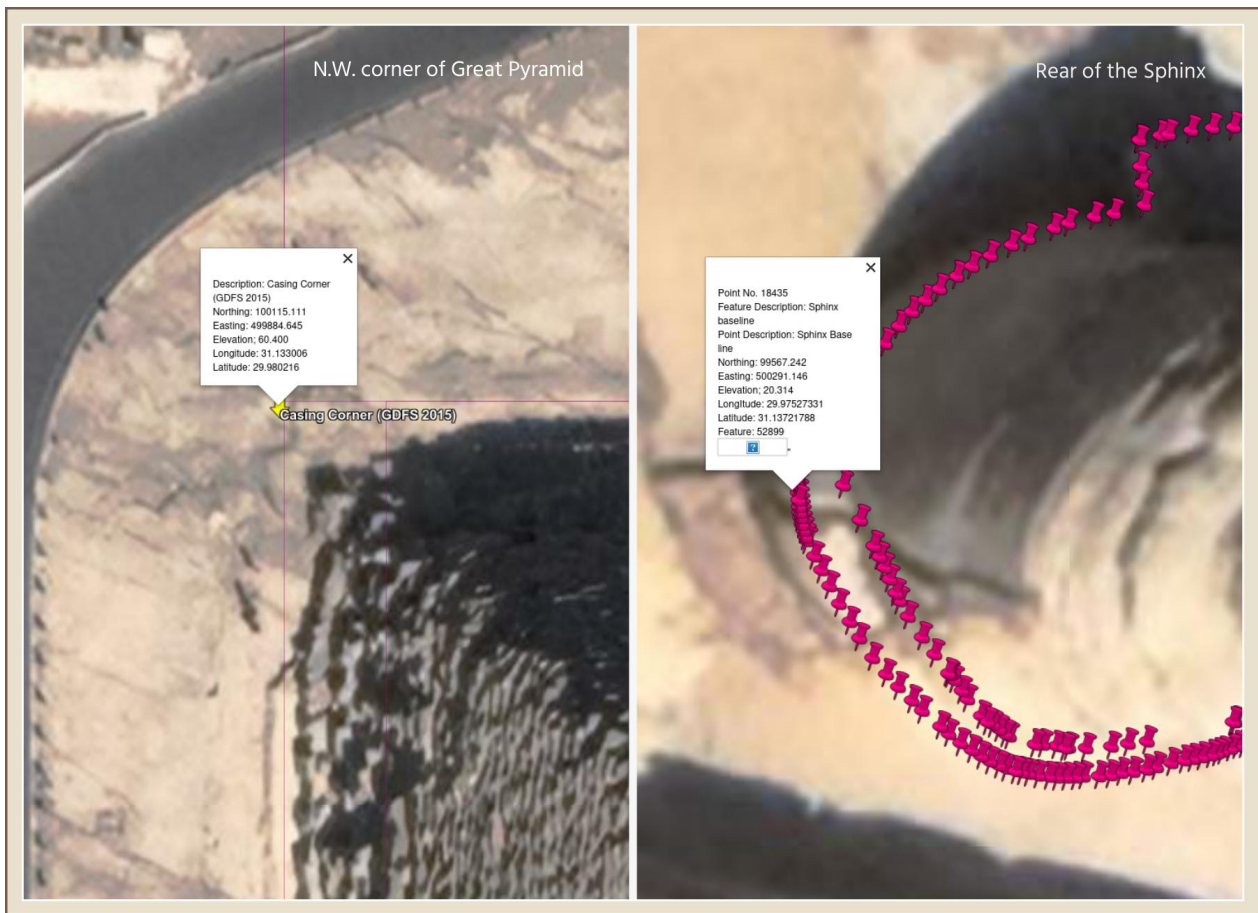
Diagram L28 - The primary surveying points on the GPMP control grid.
